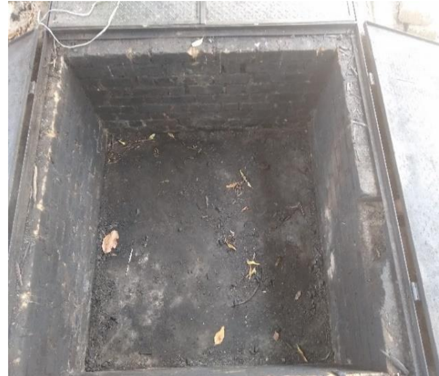
Plate 1. Customized biochar kiln used for the production of biochar
