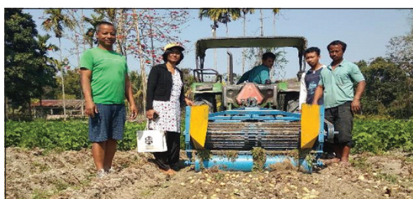
Fig. 5: Operation of potato harvester in Assam
