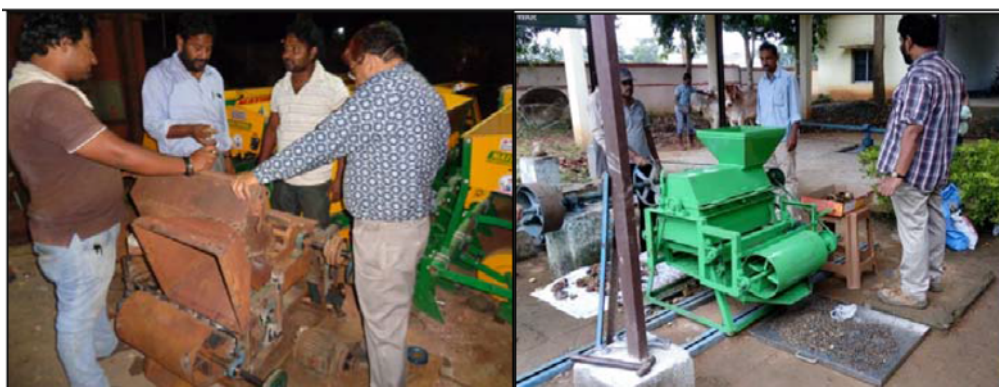
Fig. 2 : Development and evaluation of Feed in type sunflower thresher operated by bullocks in rotary mode.
